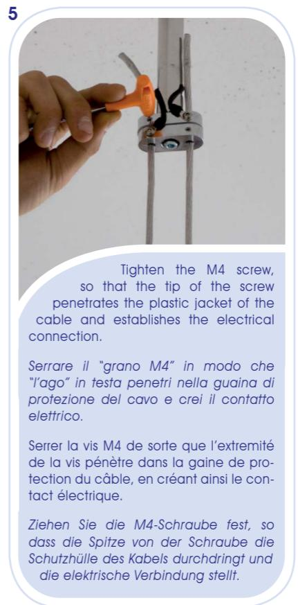
Tighten the M4 screw, so that the tip of the screw penetrates the plastic jacket of the cable and establishes the electrical connection.
